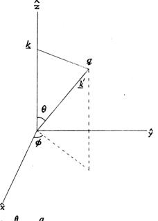
Fig. 1 Coordinate axes showing the direction of motion of the carrier along the vector  $\underline{k}$  before scattering and along  $\underline{k}'$  after scattering.
